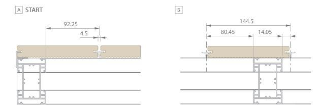
Calculate 92 mm from the edge of the first support beam (A) to the center of the joint.
