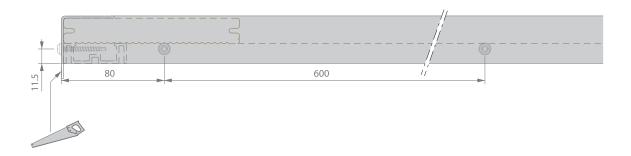
• When necessary the aluminium profile needs to be cut off in combination with the P9523 support beam.
