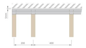
The profile can be glued or screwed on the substructure.
