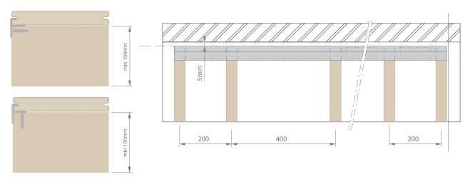
Before placing the first P 9360 Terrace plank on a Twinson, install the starter profile P 9366.
