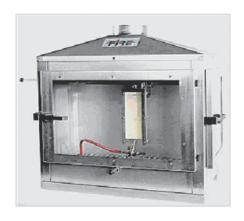
During and after the flame application it is observed whether the flame spread reaches the reference mark of 150 mm within a duration of 20 sec or 60 sec after flame application.
