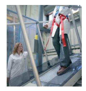
• **Barefoot Ramp Test DIN 51097**: This test is used for floor tiles or profile surfaces under wet and barefoot conditions. The tiles or profiled surfaces are fixed on a ramp which is made wet and a test operator walks on them with the ramp set at a succession of increasing angles until the person slips. The angle at which they slip is recorded. Tiles or profiled surfaces are classified into one of three groups. A, B, C, as an indication of their level of slip resistance.
