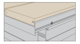
If not accesible, the profile P 9366 can be glued on the substructure. For gluing instructions see page 68.
