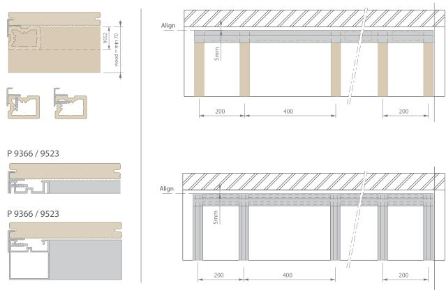
Before placing the first P 9360 Terrace plank on a Twinson or wooden substructure, install the starter profile P 9366.
