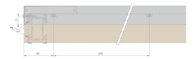
• Screwing through the Terrace Massive planks is not allowed!
